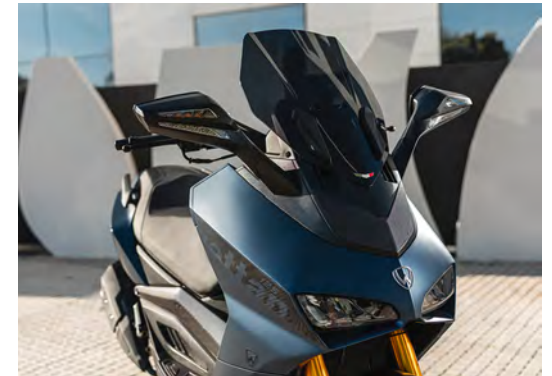
■ 5-position adjustable windscreen and integrated turn signals
