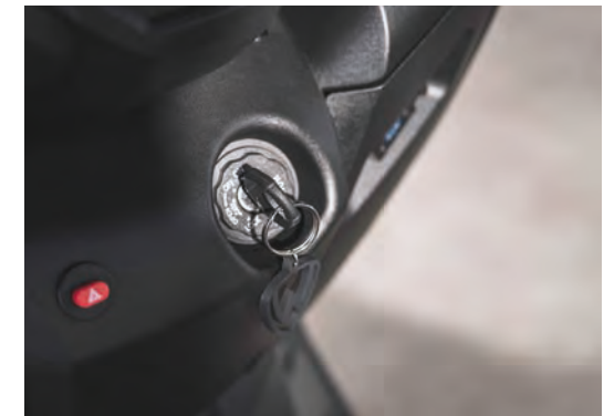
■ Locking system with seat lock and seat opening
