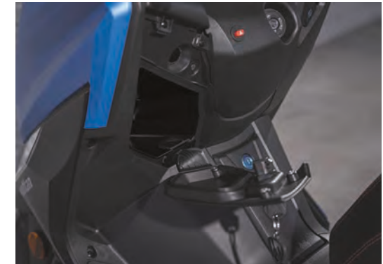
■ Two front glove compartments with USB port
